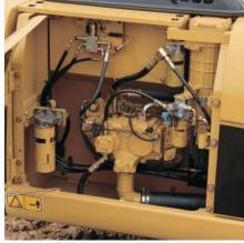
**Diagnostics and Monitoring.** The 320D is equipped with S•O•S<sup>SM</sup> sampling ports and hydraulic test ports for the hydraulic system, engine oil, and for coolant. A test connection for the Cat Electronic Technician (Cat ET) service tool is located in the cab.
